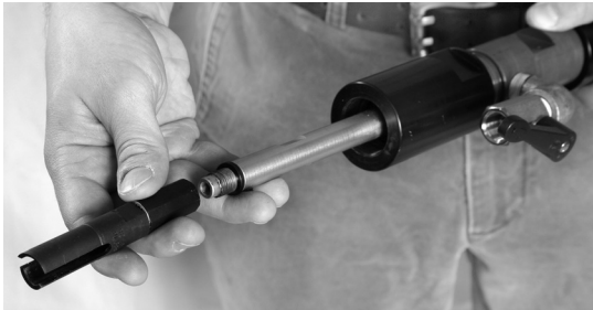
Attach coupling nut to shell cutter.
