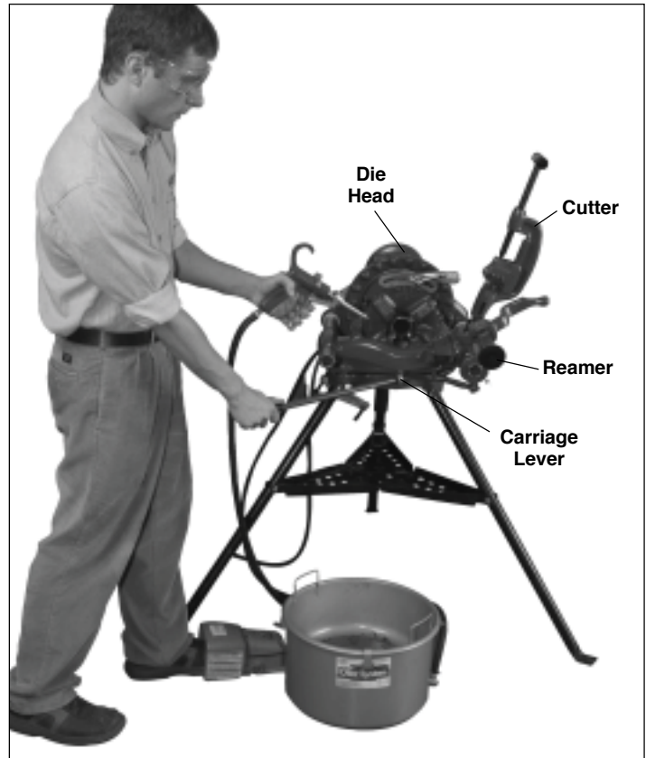
Figure 9 - Threading Pipe with R811 Die Head
