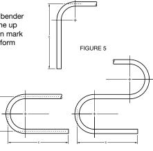
Now measure off the "X" dimension (determined in Step 2, example 3-17/32") starting from the reference mark and make a second mark (B). You are now ready to make the bends.
